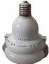
Induction lamps are ideal replacement lamps for outlawed mercury lamps in outdoor fixtures. Because they are self-ballasted, installation is simple and easy: Just screw them into existing sockets. They also offer bright white, glare-free light with a CRI above 80 for greater visibility and safety. The lamp's ballast is made of long life components that offer instant, flicker-free cold start and hot restart.
